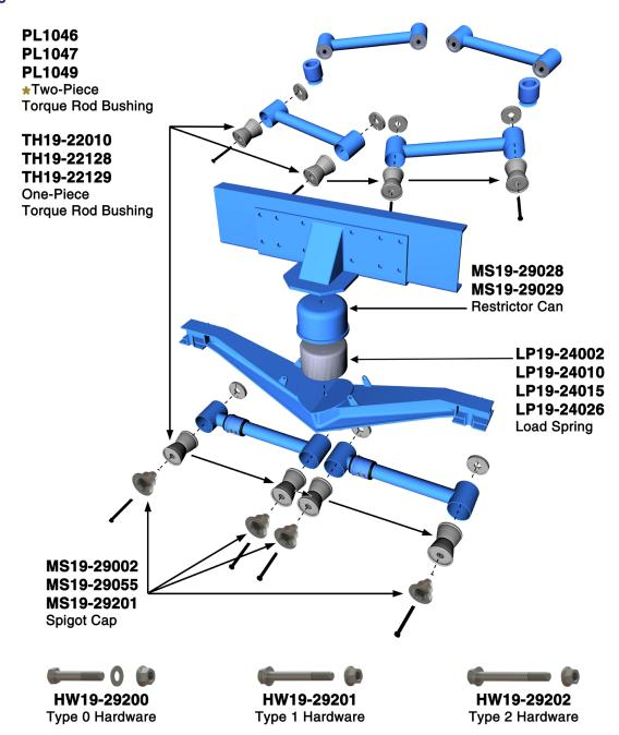
\*ATRO's two-piece bushings allow for easier installation by eliminating the interference between the spigot and ID. Simply slide one half of the two-piece bushing over opposite spigot ends and install the bare rod, install the second half of the bushings, caps and bolts. Reduces install time by 30% to 50%.
