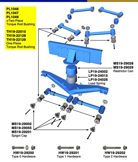
\*The ATRO two-piece design torque rod bushings allow for easier installation by eliminating the interference between the spigot and ID of the one piece bushing when installing the re-bushed torque rod. Simply slide one half of the two-piece bushing over opposite spigot ends, install the bare rod and install the second half of the bushings, caps and bolts.
