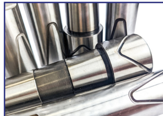
IMPROVED LUBRICATION USING ENGINEERED GROOVES ON ALL KINGPINS
